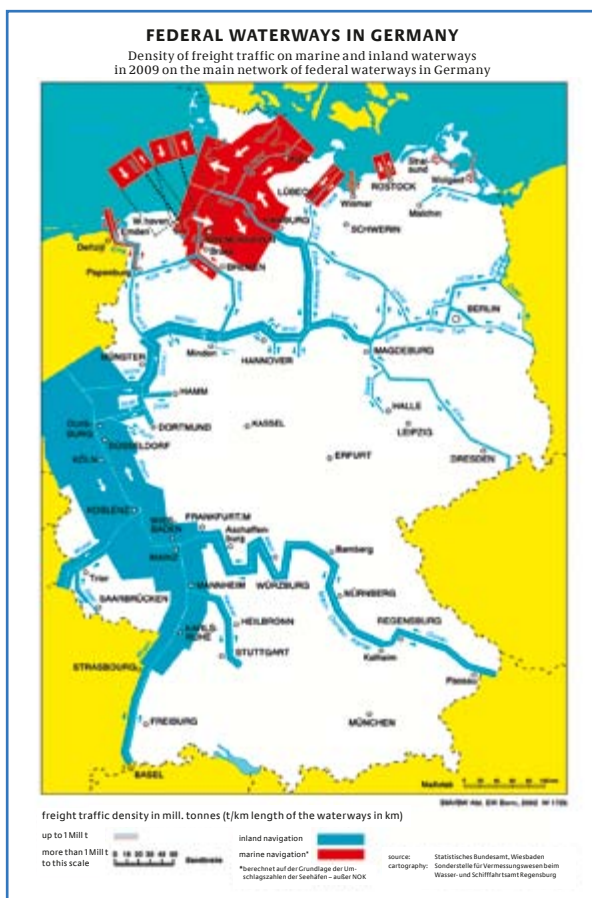
Fig. 1: Freight traffic density of marine and inland navigation on the main network of the federal waterways
